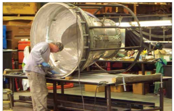
Figure 9: Preparation of an Aluminium Rotomould to Ensure a High Quality Internal Surface Finish
