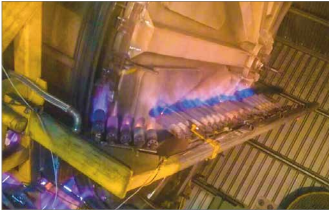
Figure 8b: Open Flame “Rock and Roll” Rotational Moulding Machine
