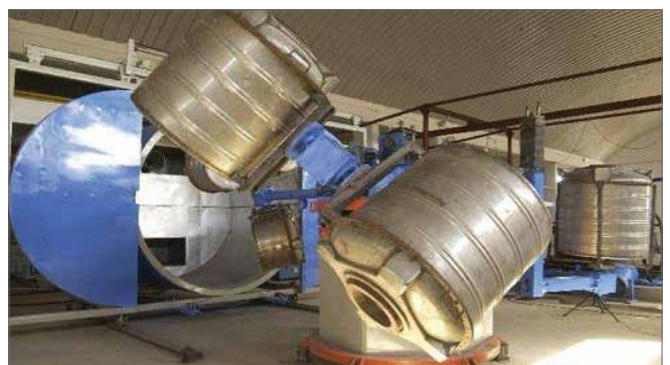
Figure 8a: Multi-Arm Rotational Moulding Machine
