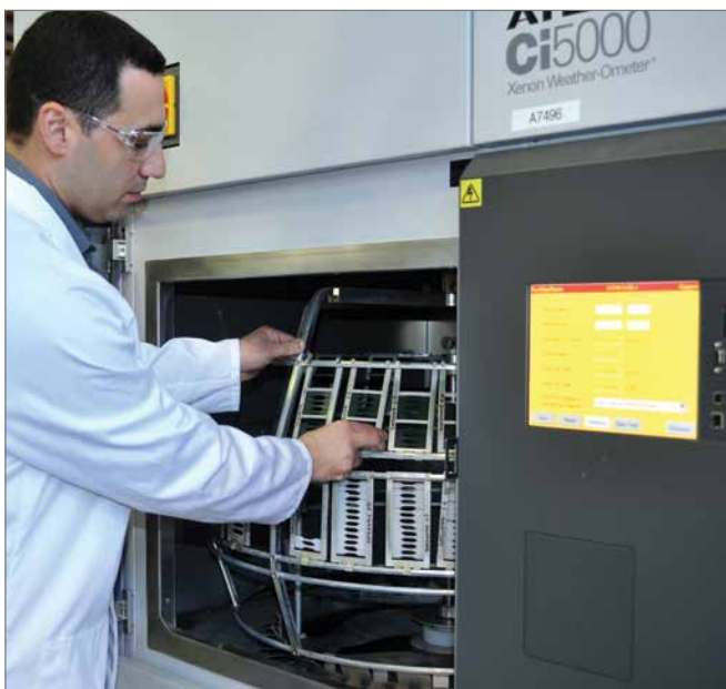
Figure 2: UV performance testing to >20,000 hours against AS/NZS 4766
